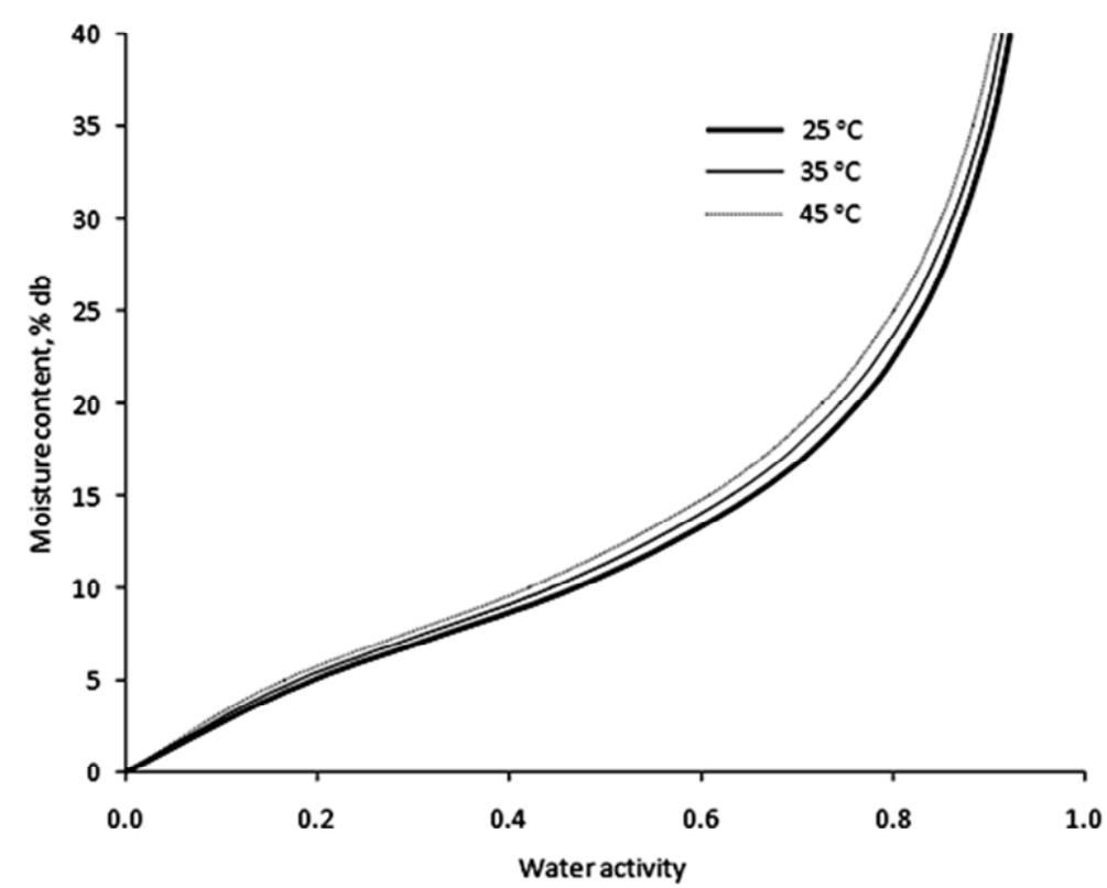
**Figure 6.** Effect of temperature on moisture sorption isotherm of sodium propionate incorporated film.
