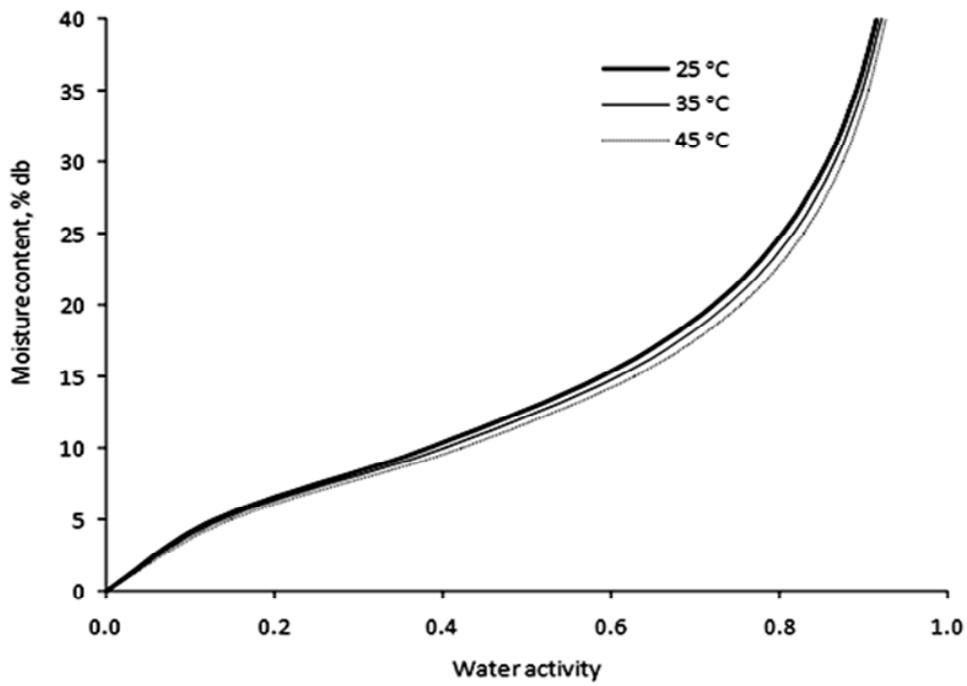
**Figure 7.** Effect of temperature on moisture sorption isotherm of benzoic acid incorporated films.
