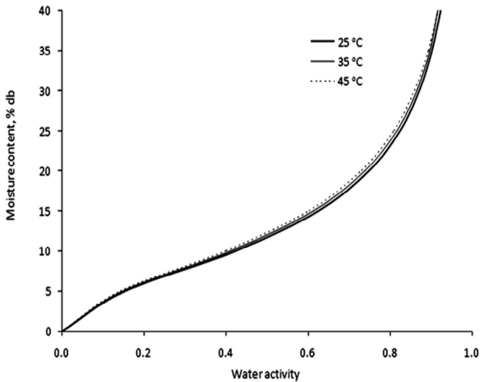
**Figure 4.** Effect of temperature on moisture sorption isotherm of control film.
