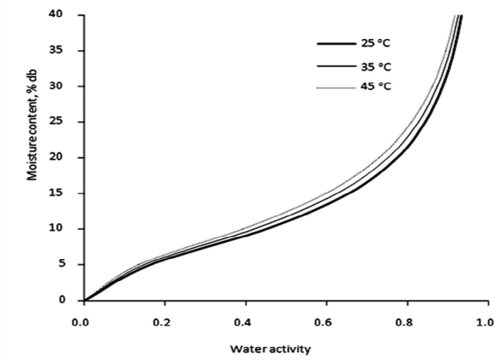
**Figure 5.** Effect of temperature on moisture sorption isotherm of potassium sorbate incorporated film
