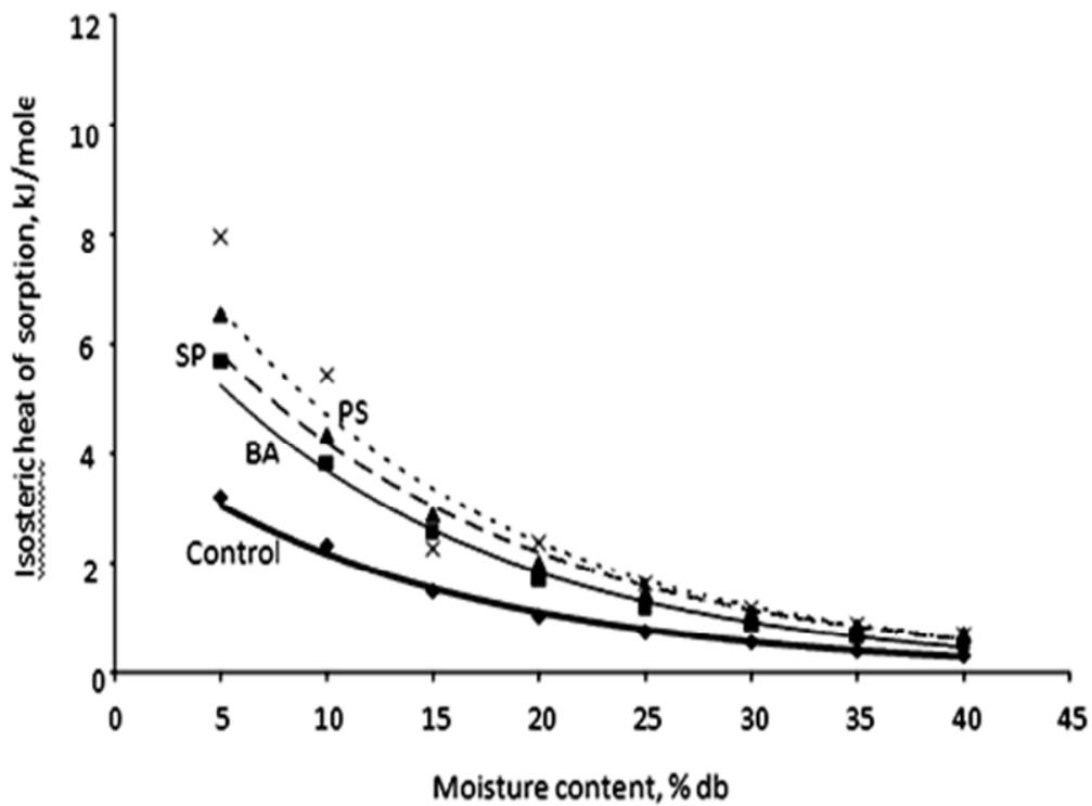
**Figure 8.** Behaviour of isosteric heat of sorption of starch based edible films at different moisture contents.
